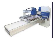
Look no further than the Bacci **MASTER CUT**, a CNC bandsaw with a router and a drilling unit, when you need a solution for cutting operations that also require millingand drilling operations. The Bacci MASTER CUT is perfect for cutting solid wood panels, MDF, plywood, plexiglass, foams and other material composites.
